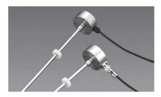
GYAF1 probe is an all-in-one sensor with the flange shape. You can get a voltage or current analog signal proportional to magnet position only by applying a 24VDC power supply directly to it. Reversed output or bipolar output can be supported as well. The flat head permits a miniaturized application, and the flange makes the installation easier, compared with the conventional screw type probes.
