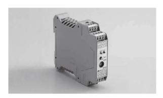
GYHC controller outputs 0–10V or 4–20mA for position and  $\pm 10V$  (or 4–20mA) for velocity. Using digital process inside, fine resolution is possible (1/65536). With option, putting 2 pcs magnets on one probe and detecting each magnet position or relative distance between 2 magnets are possible. It has toggle switches on front face for zero/gain adjustment, mounting with DIN rail. With the captive software (GPM), zero and gain adjustment is possible at user side.
