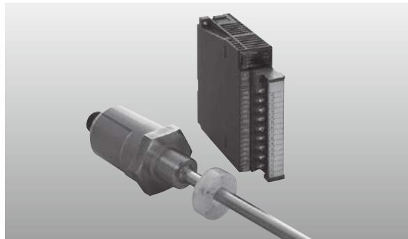
This unit is the converter for GY probe, which can be built into PLC MELSEC-Q (Mitsubishi). One unit can be associated with 1 probe (1 axis) or 2 probes (2 axes) and stores digital position data (Binary code). The CPU unit can read the data through the buffer memory.
