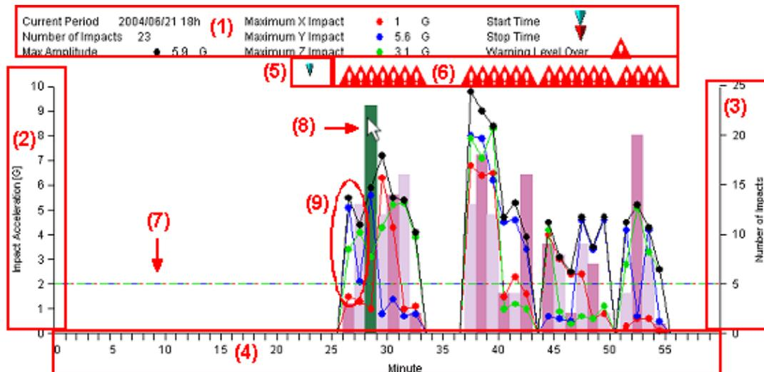
Graph displays a number of shock and magnitude. Horizontal axis of graph means time and vertical axis means magnitude and numbers of shock.
