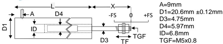
On our ACT unguided LVDTs the armature assembly is a separate component, to make a measurement the user must guide the armature inside the body without touching the sides. Our ACT unguided position measurement transducers are appropriate where external guidance is available and give truly non-contact operation
