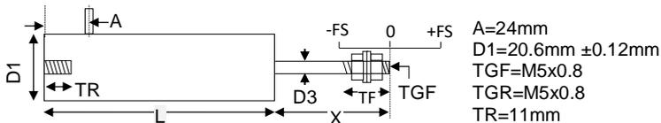
Our ACT captive guided displacement transducer has bearings to guide the armature inside the measurement sensor. Our ACT captive LVDTs are for position measurement applications where guidance may be poor and end bearings may be required.
