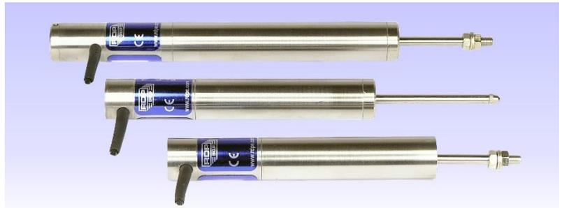
The ACT series displacement transducers form part of our industrial series of LVDTs. Because they use the LVDT principle they have a very long life as there is no electrical contact across the sensing element which means clean, reliable data. The ACT transducer gives an output proportional to the position of the armature assembly with respect to the body of the transducer. ACT series transducers are available in three versions as detailed below.
