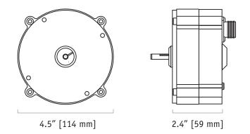
Celesco's model RT9DN communicates rotational position feedback via DeviceNET<sup>®</sup> to your programmable controller. The heart of this sensor is a precision plastic-hybrid position potentiometer which provides a "absolute" position and does not ever have to be reset to a "home" position after a power loss or planned shutdown.
