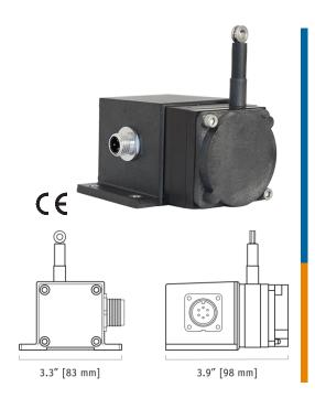
The PT1A is perfect where space and money are limited. The PT1A is part of Celesco's compact line of cable-extension transducers. Using a high cycle plastic-hybrid potentiometer, the PT1A provides a precision voltage divider position feedback signal for full-scale measurement ranges from 2 to 50 inches
