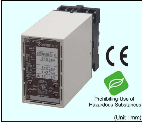
This plug-in, high-speed response type converter (isolator) provides 2 signal outputs which are mutually isolated between input, output and power-supply. It amplifies and converts various kinds of signal with isolation to use in the integrated instrumental control system. It is highly effective as noise countermeasures.
