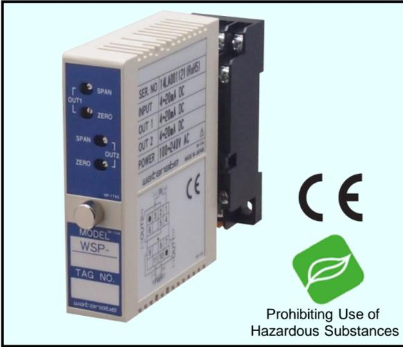
This compact plug-in signal converter connects with 3-wire type potentiometer, and provides DC voltage or current. This converter has Isolator built-in and a burnout protection circuit as standard equipment
