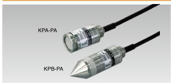
The KPA-PA and KPB-PA pore pressure gauges are used to measure pore water pressure in ground, sheet piles, piles, boreholes, etc. The KPA-PA is attached to a pile, a diaphragm wall, a sheet pile and so forth and also buried in ground to measure pore water pressure. The KPB-PA is buried in a borehole to measure pore water pressure in bedrock.
