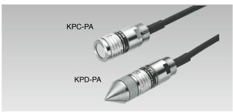
These pressure gauges, which are one size smaller than the KPA-PA and KPB-PA, are used to measure pore water pressure in soil, sheet piles, piles and boreholes. The KPC-PA is attached to a pile, a diaphragm wall, a sheet pile, etc., and buried in ground to measure pore water pressure. The KPD-PA is buried in a borehole to measure pore water pressure in bedrock.
