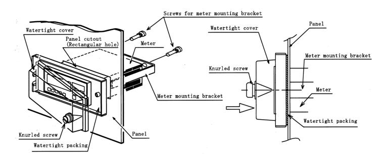
Note; After the watertight cover is mounted, check that there is no gap between the cover and panel. (As the watertight packing may deteriorate with the lapse of time, periodically check its watertightness)
