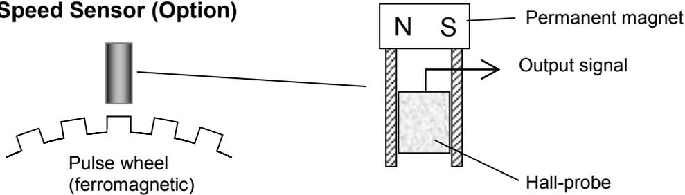
A hall sensor is located between the pulse wheel and the permanent magnet. If a tooth of the pulse wheel passes the energized hall sensor, the field intensity of the permanent magnet changes. By this, hall voltage occurs which is processed to a rectangular signal by the integrated evaluation electronics.
