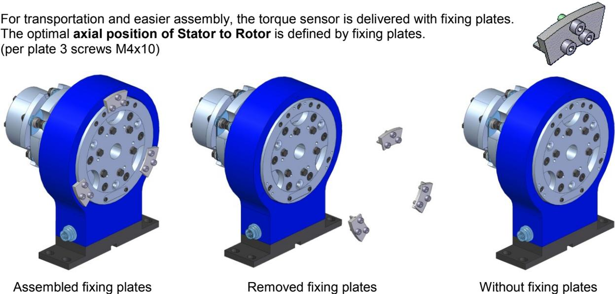
The installation and the alignment of the torque sensor occurs with mounted fixing plates. Afterwards remove the 3 fixing plates and control position of shaft to stator:
