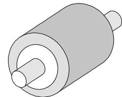
Shift couplings on shafts (use entire clamping length of the coupling) and align shafts.
