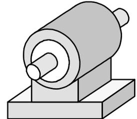
Shafts have to be cleaned with solvent (e.g. acetone) before the assembly
