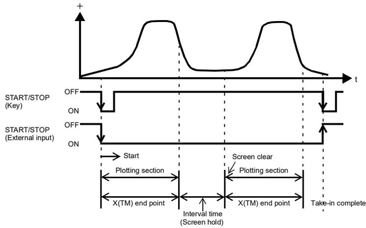
Continued Trigger: Plots a graph continuously using the trigger.
