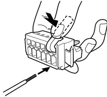
The wire can be connected likewise without the operating tool by using a tool such as a flathead screwdriver to press down the spring from the top.
