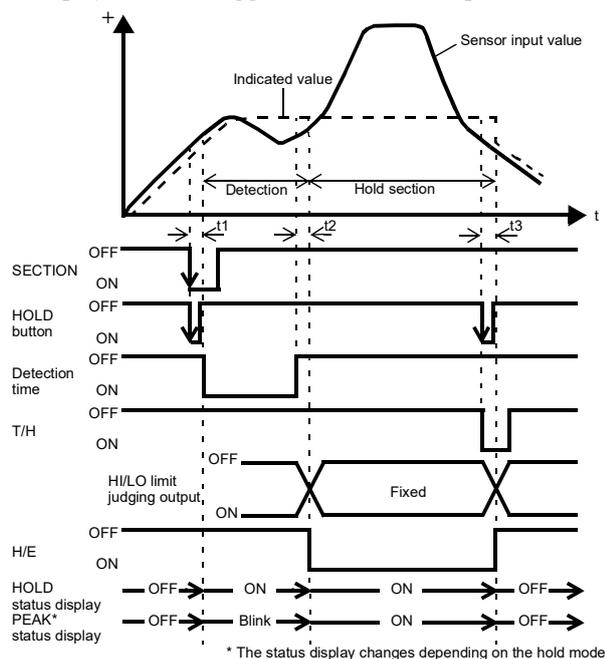
t1: A delay time between the instant when the SECTION signal is inputted and the instant when the value to be held is detected
