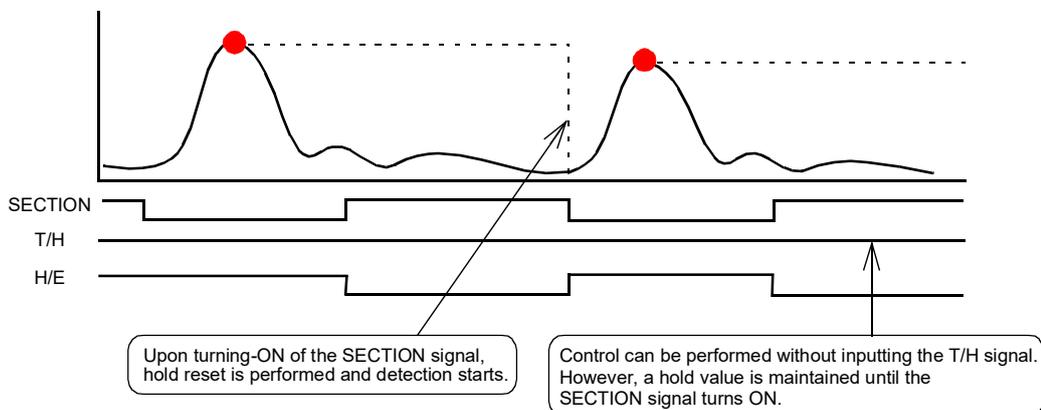
However, when the auto reset functions, if the signal causes chattering, the point that should be taken originally may deviate. Switching is provided so as to prevent the next detection from being performed until the T/H signal is turned on even if the SECTION signal is turned on again.
