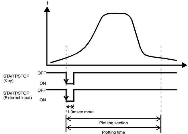
Single Trigger: Plots a graph only once using the trigger.
