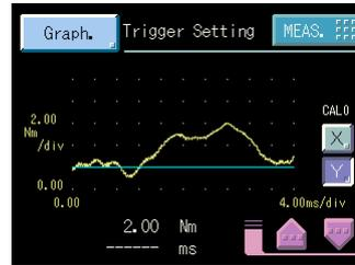
Setting using a numerical value as a pre-trigger value is also possible.
