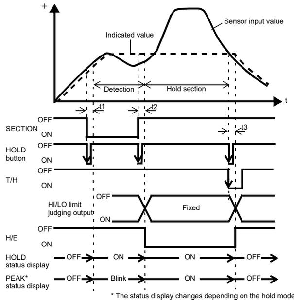
t1: A delay time between the instant when the SECTION signal is inputted and the instant when the value to be held is detected
