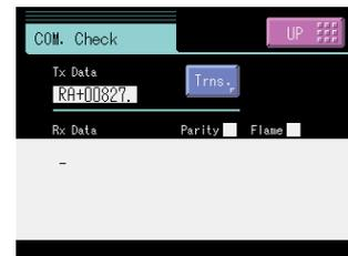
Please transmit something information sentence from connected equipment side to the check on the reception. The data received to "Receive data" is displayed. Please confirm the cable or the setting of communication condition when it is not correctly displayed, when "Parity" or "Frame" lights in red.
