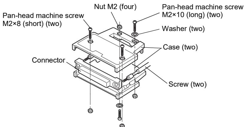
1. Set the connector and screws (two) into the grooves of the case (one side).
