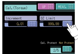
4. Enter the digital zero limit value by the numerical keys and determine with the [OK] button.
