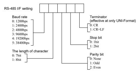
**2.** Make initial settings of the RS-485 port of the personal computer, PLC, etc., connected according to the settings of this device.
