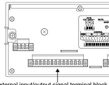
External input/output signal terminal block
