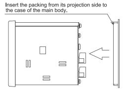
**3.** Insert the projection of the packing all around the clearance of the front panel.
