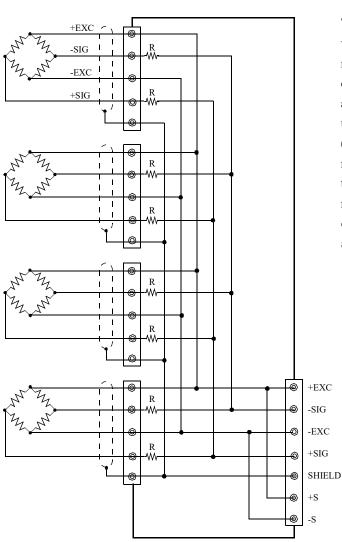
The group of "n" parallel load cells viewed from this device side can be regarded as a unit load cell the rated capacity of which is multiplied by "n" and the sensitivity of which is unchanged. The averaging resistance (R) should be  $300 - 500\Omega$ , equal in relative ratio and excellent in temperature coefficient. No averaging resistance is needed if load cells with consideration for parallel connection are used.
