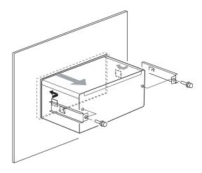
**4.** Securely fix the mounting hardware on both sides with the attached M4 screws.
