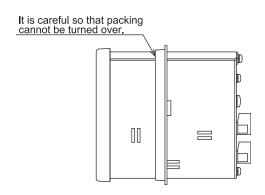
**4.** Check that there is no gap or twist between the inserted packing and front panel. If there is a gap, push in the packing to bring them into close contact.
