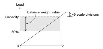
For accurate span calibration, it is recommended to perform it with the balance weight value between 50% and 100% of the capacity.
