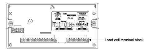
Load cell terminal block pin assignments
