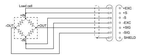
Remote sense lines are used to detect and correct variations in excitation voltage over long cable runs.
