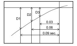
You can insert the digital filter to restrain the weight value from fluctuating when the stable signal is ON.
