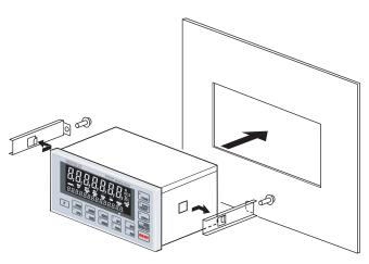
3. Insert the mounting rails into both sides from the back of the indicator.
