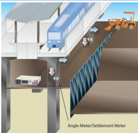
Deformation measurement in neighboring construction
