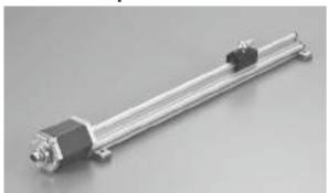
This is the linear profile version of GYSE-S. GYSE-S probe outputs displacement of the magnet as SSI (Synchronous Serial Interface). SSI is output of a serial communication-type and outputs the position data of 24 - 27 bit. When using SSPC-03 of separate sale, you can convert SSI to parallel data. So you can get the data in the I/O unit. The inside probe element can be detached from the outer housing, and with the captive software (GPM), zero and gain adjustment is possible at user side.
