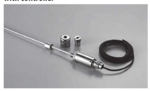
EX-GYdT-R probe is a level or displacement transducer of the flameproof enclosure type which has GYcRS circuit inside. Having the closed structure for sensor head achieves waterproof performance and compact. An explosion protection symbol is Exd II CT6, and you can use it in the most of the explosive gas atmosphere.
