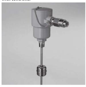
EX-GYdS-R probe is a level or displacement transducer of the flameproof enclosure type which has GYcRP circuit inside. An explosion protection symbol is Exd II CT6, and you can use it in the most of the explosive gas atmosphere.
