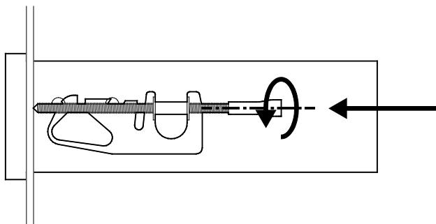
4. Turn the set screw with a blade screwdriver to the stop on the front plate.
