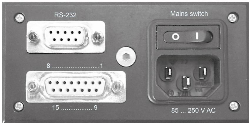
Wiring of connector X1 see table “Wiring basic unit”.
