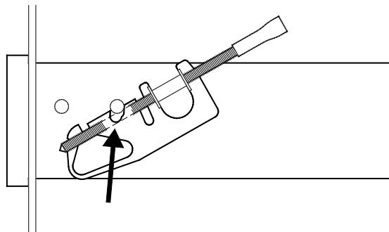
2. Hook the mounting clamp to the rear notch.
