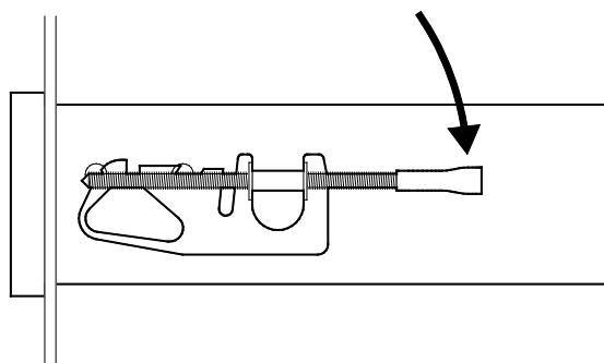
3. Push down the end of the mounting clamp until the front notch is locked.
