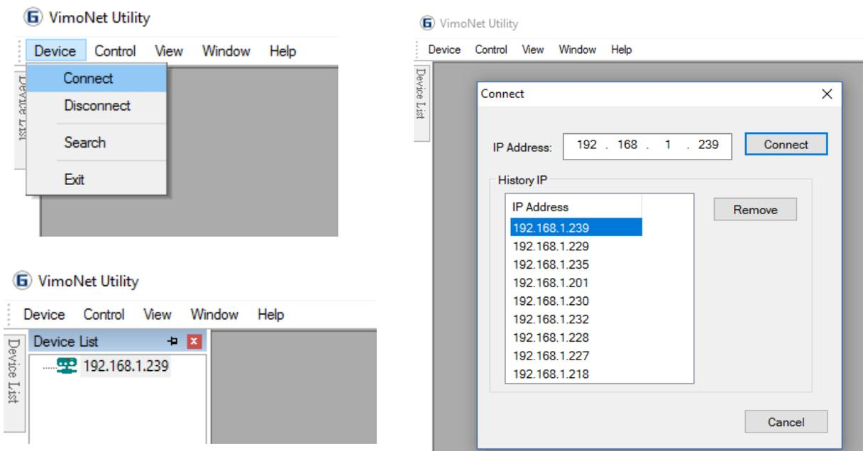
Figure4.4 Connect devices through IP address
