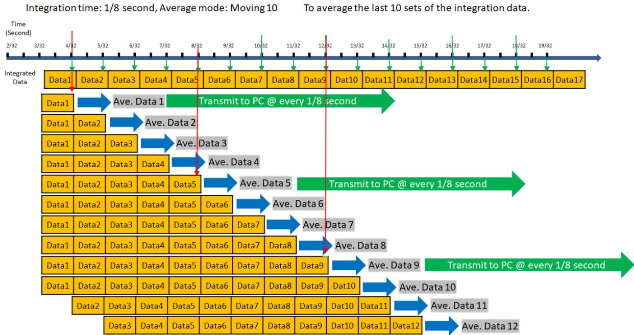
Figure4.13 Integration time: 1/8 second, Average mode: Moving 10
