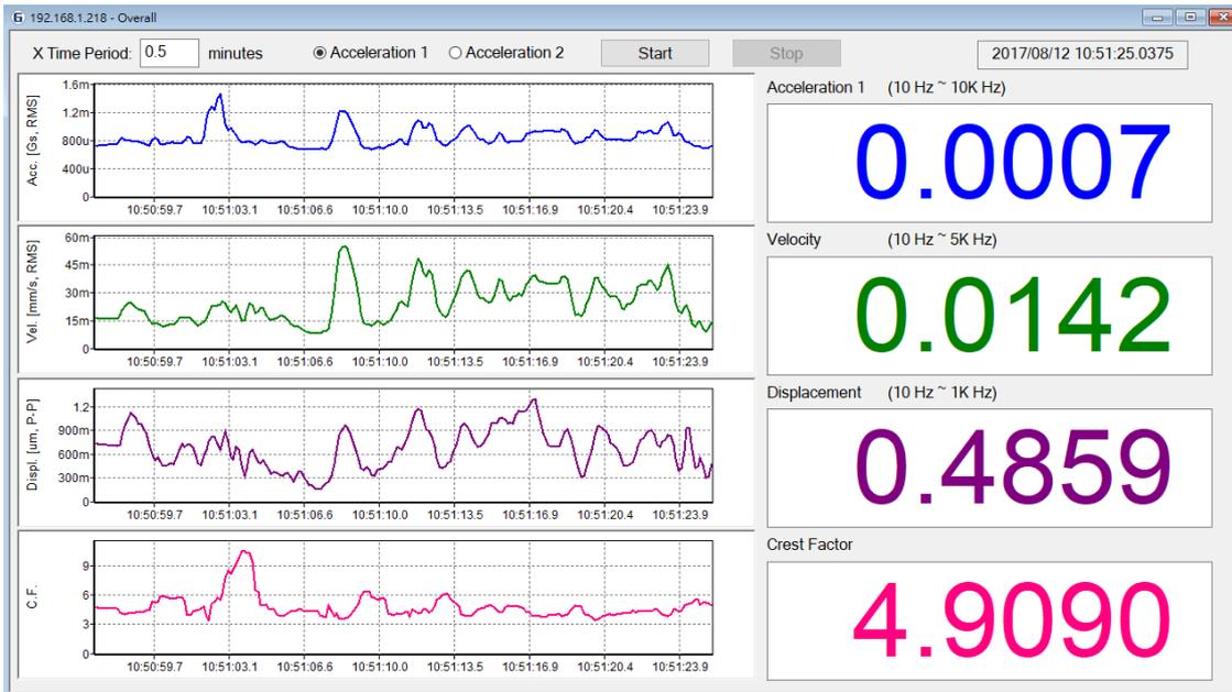
Figure4.14 Vibration value is stable @ Integration time: 1/8 second, Average mode: Moving 10
