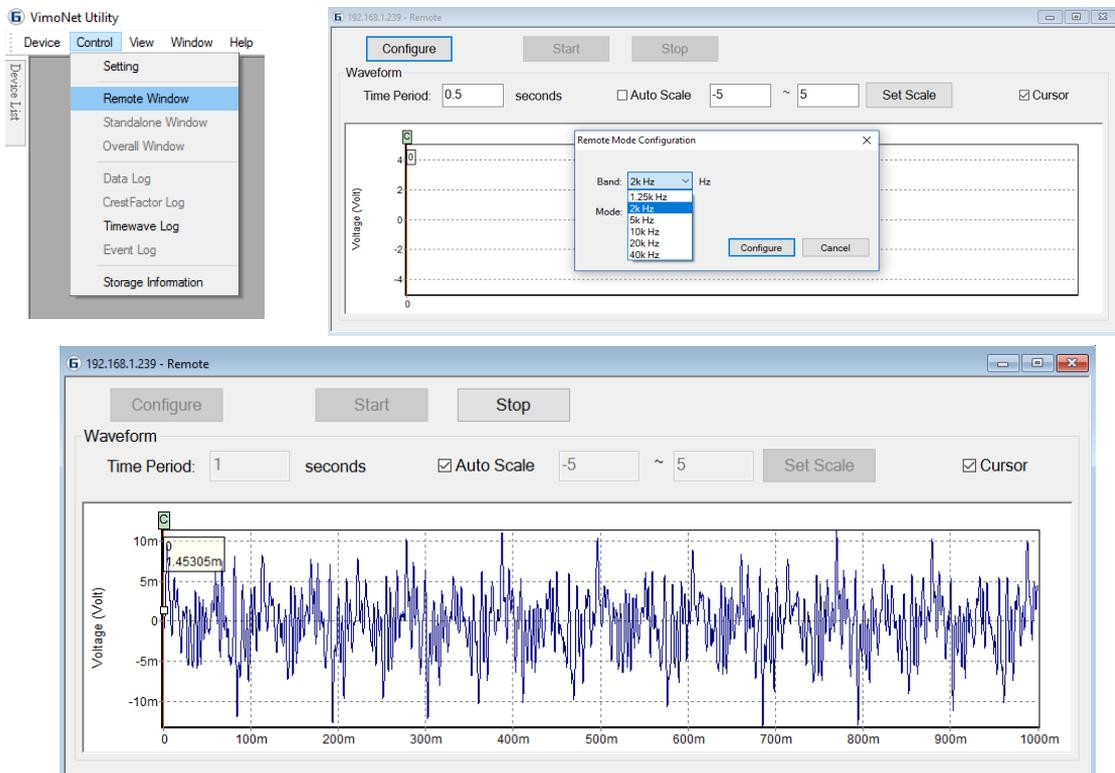
Figure4.18 Remote mode setting and display
