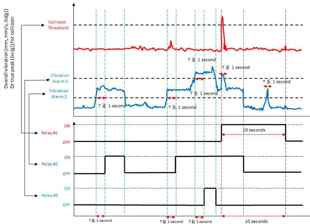
Figure4.16 Relay triggered condition and sequence
