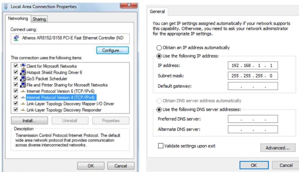
Figure3.3 IP address and setting
