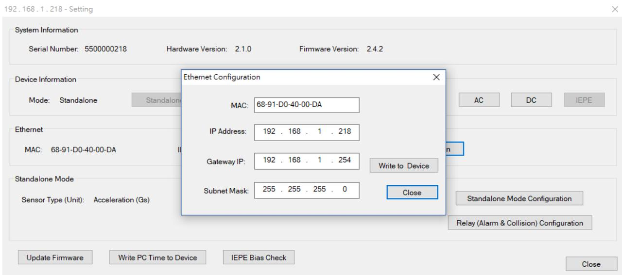
Figure4.6 Control/ Setting/ Ethernet Configuration window
