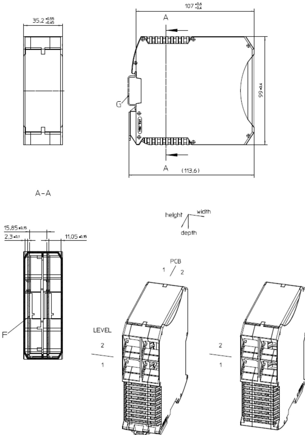
Figure2.3 Dimension of the device case
