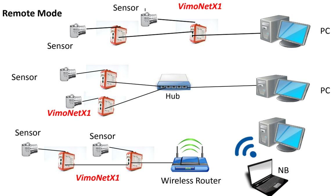
Figure2.2 Remote mode system configuration
