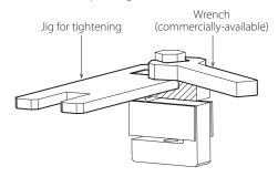
• In the same way, when attaching a rod end or base, for example, to the screw/bolt area on the bottom of the load cell, use the included jig to hold the area shown with diagonal lines at the bottom and tighten the screw or nut.
