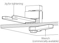
• When tightening the screw or nut attached to the load cell, holding the screw/bolt part on the opposite end (shown with diagonal lines), will cause twisting force to be applied to the gauge and break the load cell.
