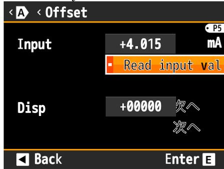
●Operation for full scale calibration (ex: InputRange 4-20mA, set display value to be 0-10000)
