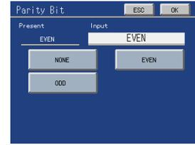
Main screen→Setting→First Setting→Com. Setting→Parity Bit
