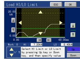
Main screen→Setting→Work Setting→Hold Setting→Load HI/LO Limit
